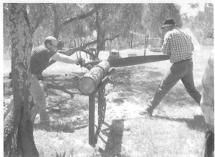
A demonstration of using a cross-cut saw.
